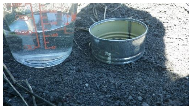
1 Measured water and ring pounded into ground ready to pour and time
