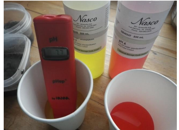
2Using buffer solutions to calibrate pH meter
